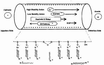
Fig. 9 Pictorial Diagram of Indirect UV Detection
